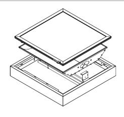
To replace the light source it is necessary to take out perforated mesh(optionally louver)
