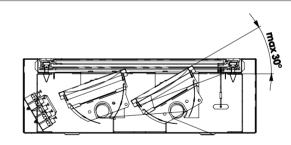
To replace the light source it is necessary to take out perforated mesh(optionally louver) Louvers are mounted independently on swinging pans and the rest on springs. Each louver can be adjusted of angle max 30 degrees In order to replace the fluorescent lamp it is necessary to take out the louver with the pan.
